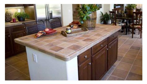
Tiles can be made from ceramic, porcelain or natural stone. Ceramic tiles are made from pressed clay. They come in matte, metallic or glazed finishes. Glazed finishes are more susceptible to scratches. Porcelain tiles, also made from clay, are baked at high temperatures and hide scratches and chips better than ceramic tiles because the colour goes through the full thickness of the tile. To reduce staining of the grout on your tile countertop or backsplash, apply grout sealer every other year.
